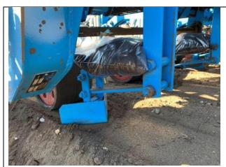
Weight on the plough (sandbag) to ensure that the plough does not slide on top of the solid soil but pushes the soil to the sides at uniform depth. A primitive solution to a difficult practical problem.
