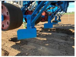
Front plough lowered so that it presses into loose soil and pushes it to the sides before the front wheel.
